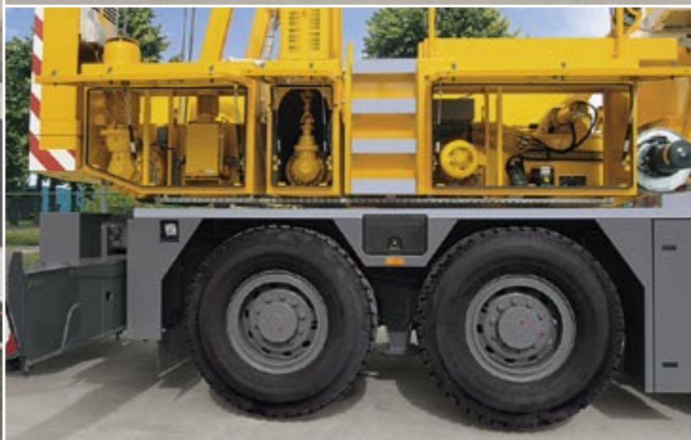
The drive assemblies are easily accessible for servicing.
